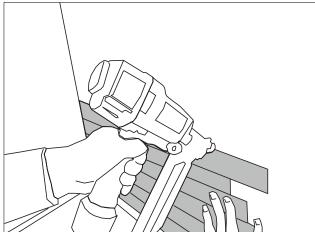
Checking to make sure you are keeping the plank straight, continue nailing the plank until you get to the end of the plank. For nail/staple installations to furring strips, planks will need to be cut to ensure that ends land on the furring strip. This is not necessary when installing over plywood sheathing.
